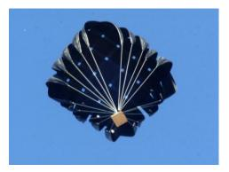
The **High-Velocity parachute**, which will be the low-cost replacement for the existing 26-foot ringslot parachute, is made of lengths of woven polypropylene material sewn at the crown in a cross-hatch pattern, with nylon suspension lines to attach to the containerized load.
