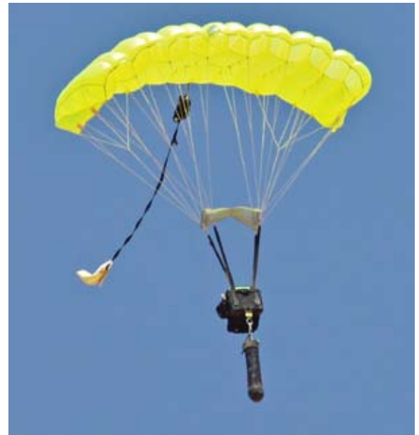
Onyx ML system with mock sensor payload
