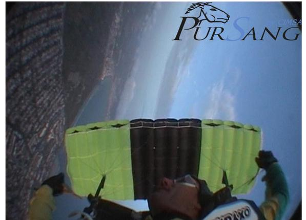
Pursang is the first canopy in the world that incorporates the new Synchronized Inflow Control System SICS® to control the inflation process during deployment. This innovative system developed by CIMSA Ingeniería de Sistemas results in very soft and straight canopy deployments even in very high wing loading conditions.
