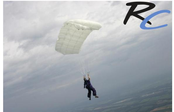
The RC exceeds the requirements of the Aerospace Standard AS8015B, the FAA TSO-C23d and the EASA ETSO-C23d. Its rugged construction uses additional reinforcement chord wise, span wise, throughout the nose, and at all line attachment points.
