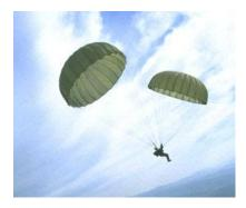
The 24-foot Diameter Chest Reserve Assembly is an emergency parachute designed to be used in the event of a malfunction of the primary back type parachute.
