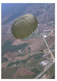
This change reduced the opening shock by providing a slightly larger diameter at the skirt hem; providing a lower rate of descent and a softer landing. All T-10B Canopies in service have now been upgraded to the new Pocket Band length.
